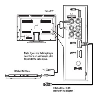
3 If you are connecting a DVI device, connect an audio cable with stereo mini plug (not provided) to the L and R AUDIO jacks on the side of your TV and to the AUDIO OUT jack on the DVI device.
